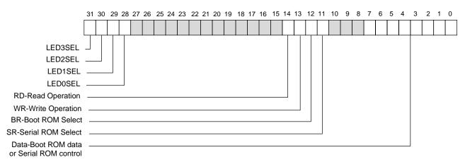
Field Name Description 31 LED3SEL 0:Default value. Set LED3 as RX LED. 1: Set LED3 as Full/Half duplex LED. LED2SEL 0:Default value. Set LED2 as Link Speed (10/100) LED. 30 1: Set LED2 as Collision LED. 29 LED1SEL 0:Default value. Set LED1 as Good Link LED. 1: Set LED1 as Link/Activity LED. 0:Default value. Set LED0 as Activity LED. 28 LED0SEL 1: Set LED0 as Link Speed (10/100) LED. RD Boot ROM/EEPROM read operation select bit. 14
