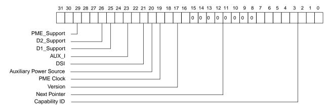
bit 31-27 : PME\_Support, read only indicates the power states in which the function may assert PMEB pin.
